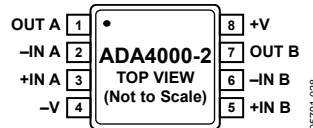
Figure 4. 8-Lead MSOP (RM-8)
