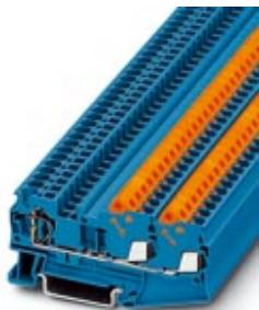
Feed-through terminal block, Connection type: Quick connection, Spring-cage connection, Cross section: 0.5 mm<sup>2</sup> - 2.5 mm<sup>2</sup>, AWG :20- 14, Width: 6.2 mm, Color: blue, Mounting: NS 35/7,5, NS 35/15
