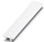
Zack marker strip, Can be ordered: Strip, white, Labeled according to customer specifications, Mounting type: Snap into tall marker groove, For terminal block width: 6.2 mm, Lettering field: 6.15 x 10.5 mm
