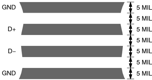
Figure 21. Typical Arrangement of Signal Tracks
