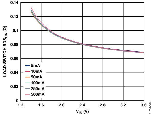
Figure 4. Load Switch RDS<sub>ON</sub> vs. Input Voltage ( $V_{IN}$ ) for Different Load Currents
