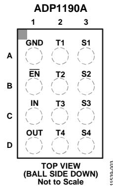
Figure 3. Pin Configuration
