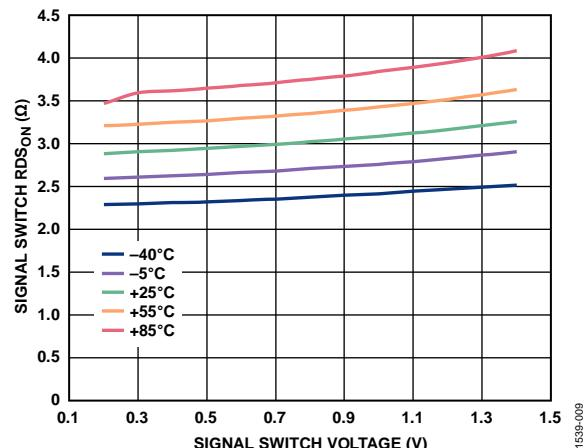
Figure 9. Signal Switch RDS<sub>ON</sub> vs. Signal Switch Voltage for Various Temperatures,  $V_{IN} = 1.4\text{ V}$
