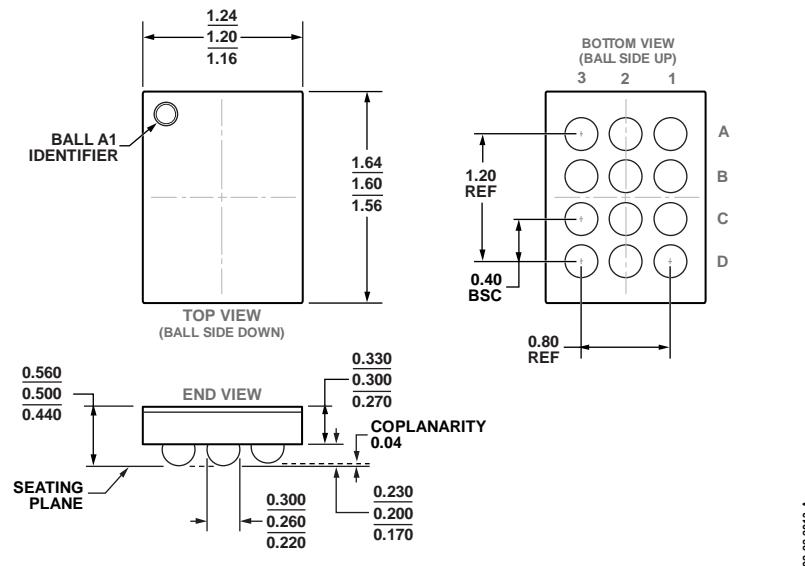
Figure 24. 12-Ball Wafer Level Chip Scale Package [WLCSP]
