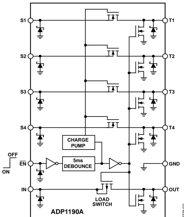
Figure 21. Block Diagram with ESD Protection Devices
