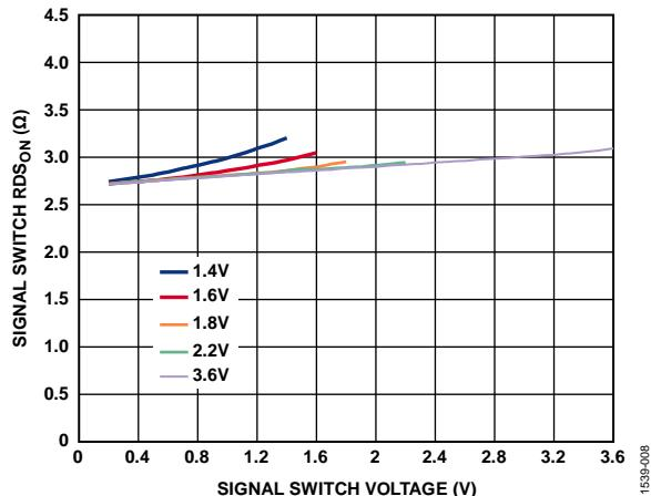
Figure 8. Signal Switch RDS<sub>ON</sub> vs. Signal Switch Voltage, Different Input Voltages
