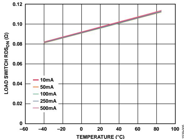
Figure 5. Load Switch RDS<sub>ON</sub> vs. Temperature for Different Load Currents,  $V_{IN} = 1.8\text{ V}$
