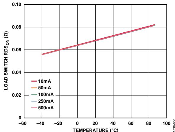
Figure 6. Load Switch RDS<sub>ON</sub> vs. Temperature for Different Load Currents,  $V_{IN} = 3.6\text{ V}$
