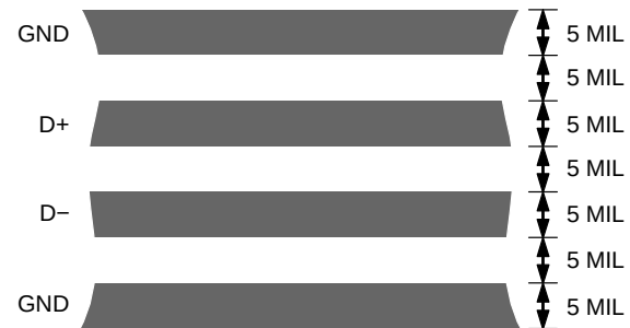
Figure 12. Typical Assignment of Signal Tracks
