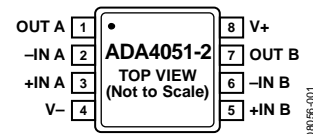
Figure 3. 8-Lead MSOP (RM-8)
