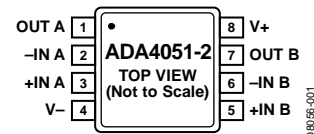
Figure 3. 8-Lead MSOP (RM-8)
