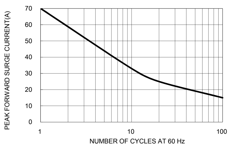
FIG. 2 MAXIMUM FORWARD SURGE CURRENT
