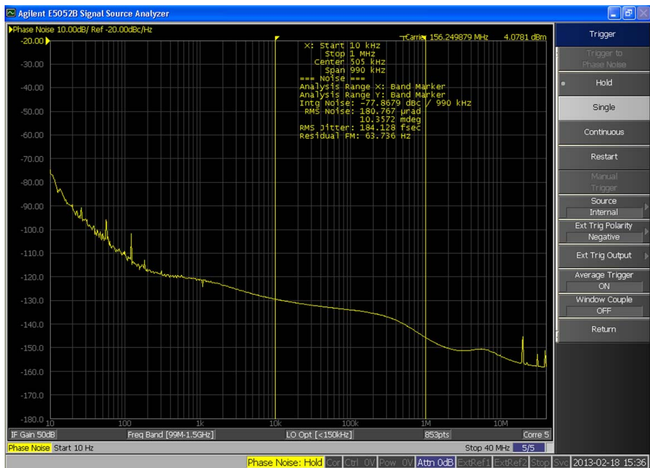
Figure 1. Si535/536 Typical Phase Noise at 156.25 MHz
