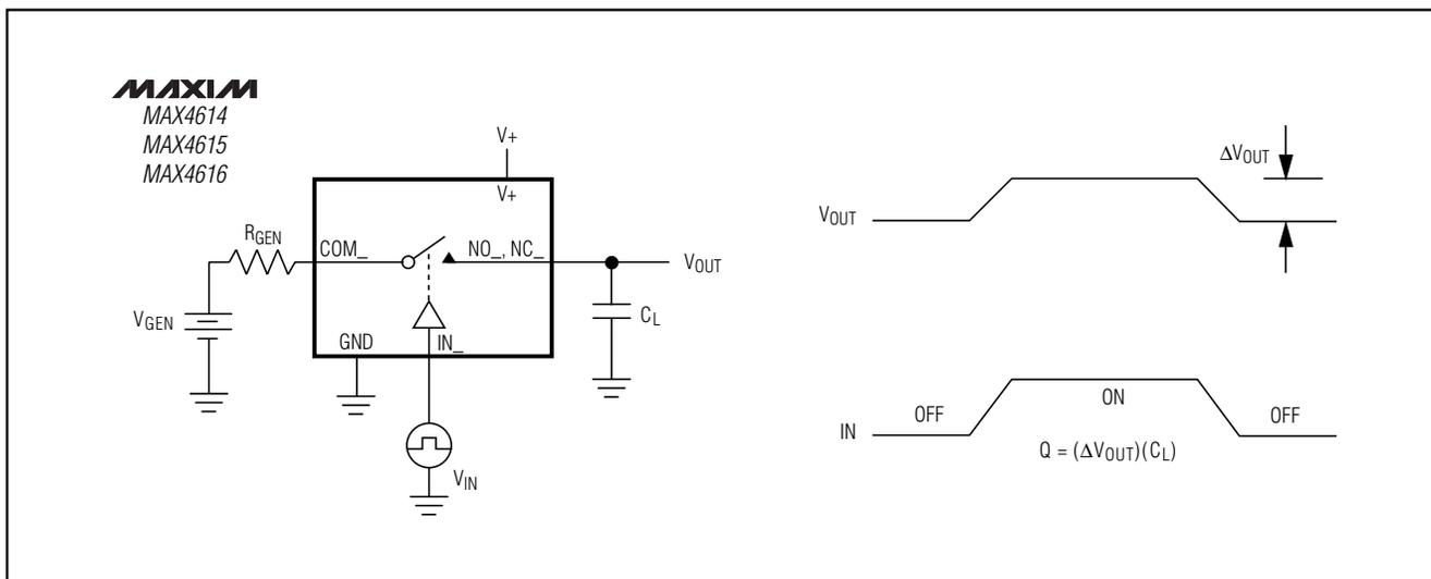
Figure 3. Charge Injection
