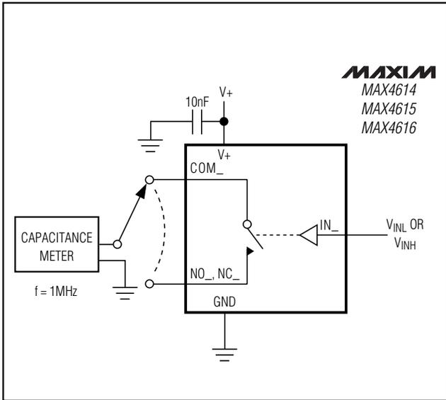
Figure 6. Channel Off/On-Capacitance
