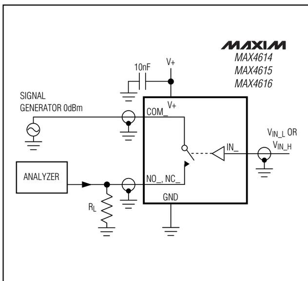
Figure 4. Off-Isolation/On-Channel Bandwidth
