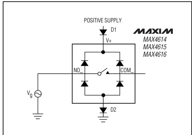
Figure 1. Overvoltage Protection Using Two External Blocking Diodes
