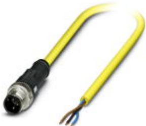
Sensor/Actuator cable, 3-position, PVC, Yellow RAL 1021, Plug straight M12-SPEEDCON, A-coded, on Free cable end, Cable length: 2 m
