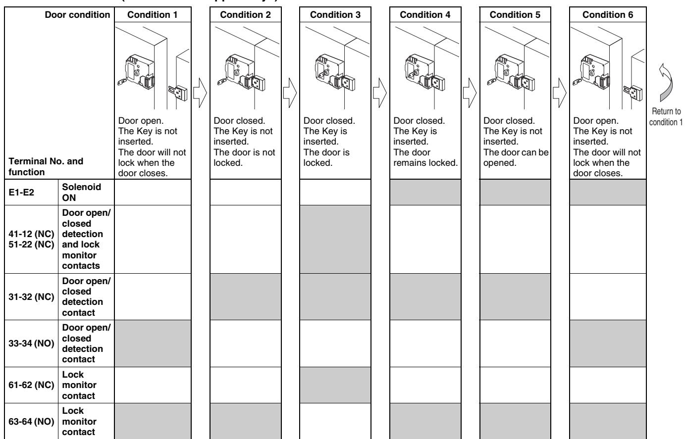
The shaded areas indicate the contact is closed and power is supplied to the solenoid.
