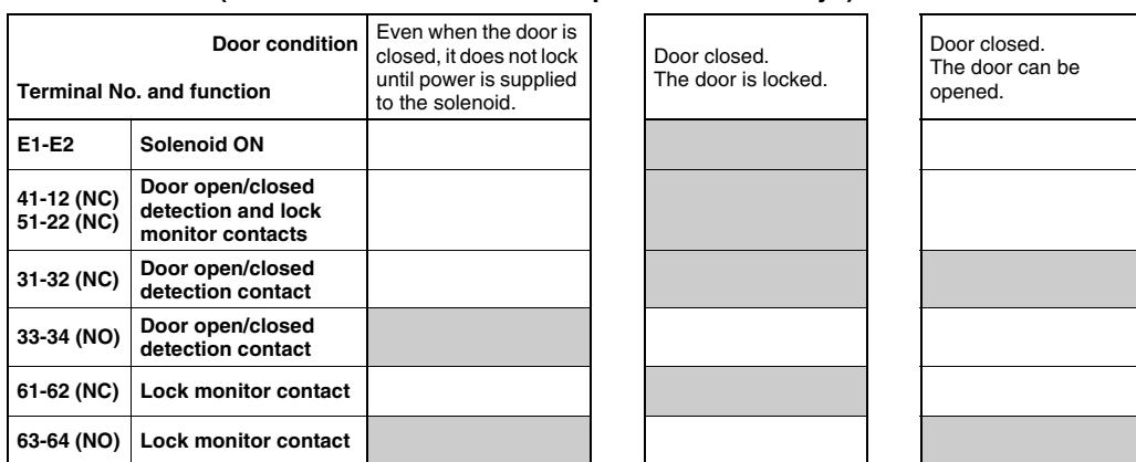
The shaded areas indicate the contact is closed and power is supplied to the solenoid.
