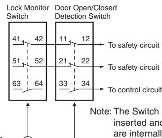
Note: The Switch is shown with the key inserted and locked. Terminals 42 and 11 are internally connected, as are terminals 52 and 21 (according to GS-ET-19).
