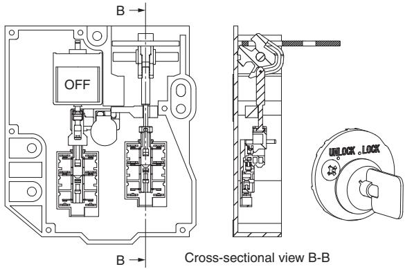
(6) Operation Key removed, solenoid ON, and trapped key removed.
