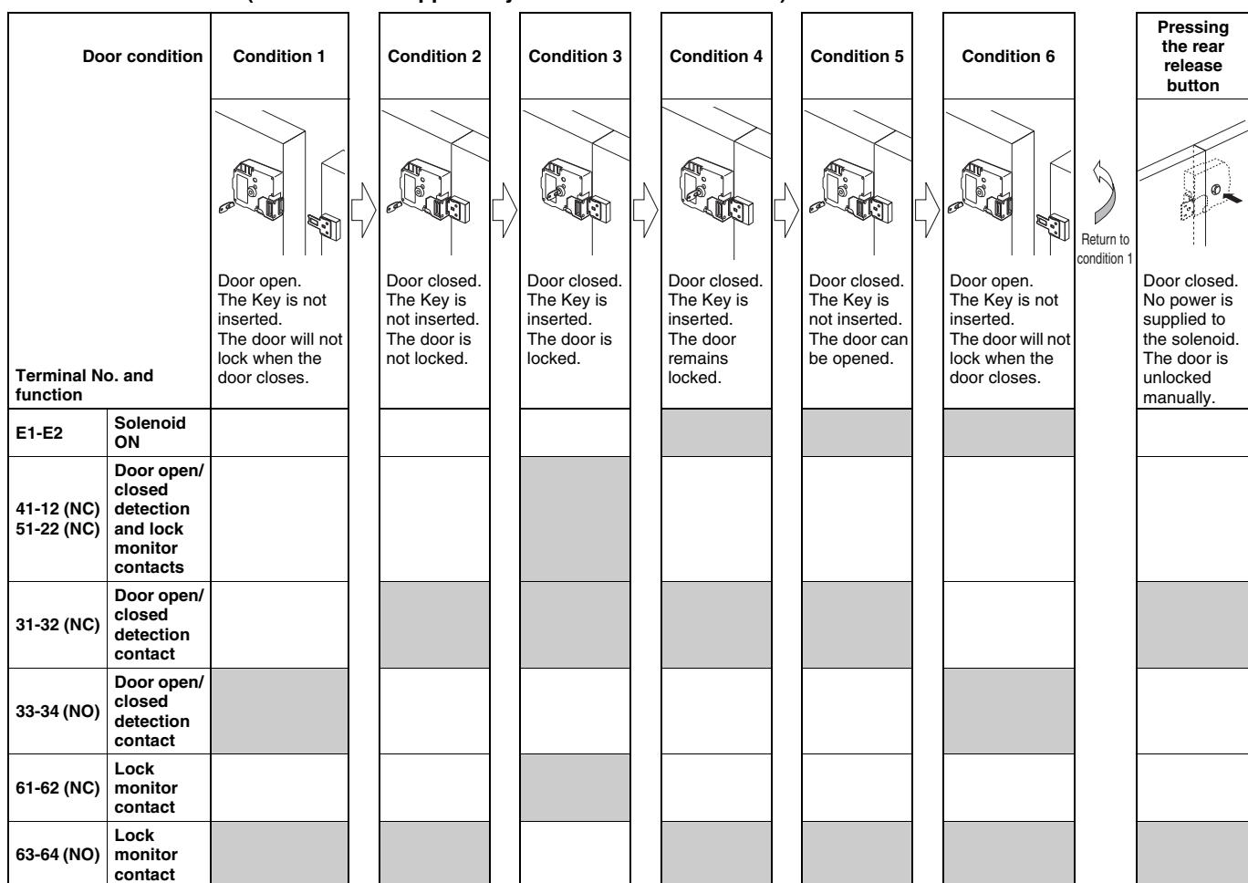
The shaded areas indicate the contact is closed and power is supplied to the solenoid.
