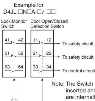
Note: The Switch is shown with the key inserted and locked. Terminals 42 and 11 are internally connected, as are terminals 52 and 21 (according to GS-ET-19).
