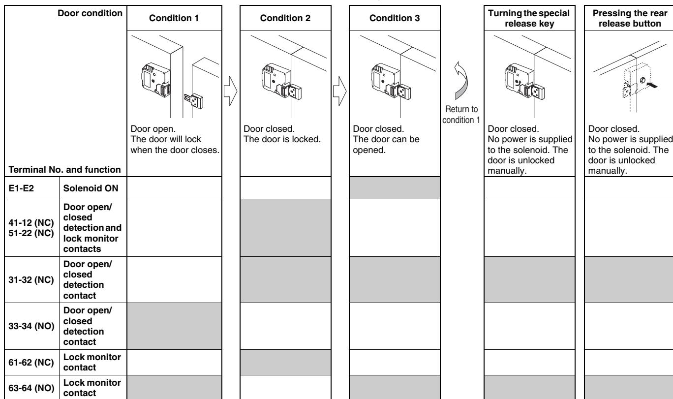
The shaded areas indicate the contact is closed and power is supplied to the solenoid.
