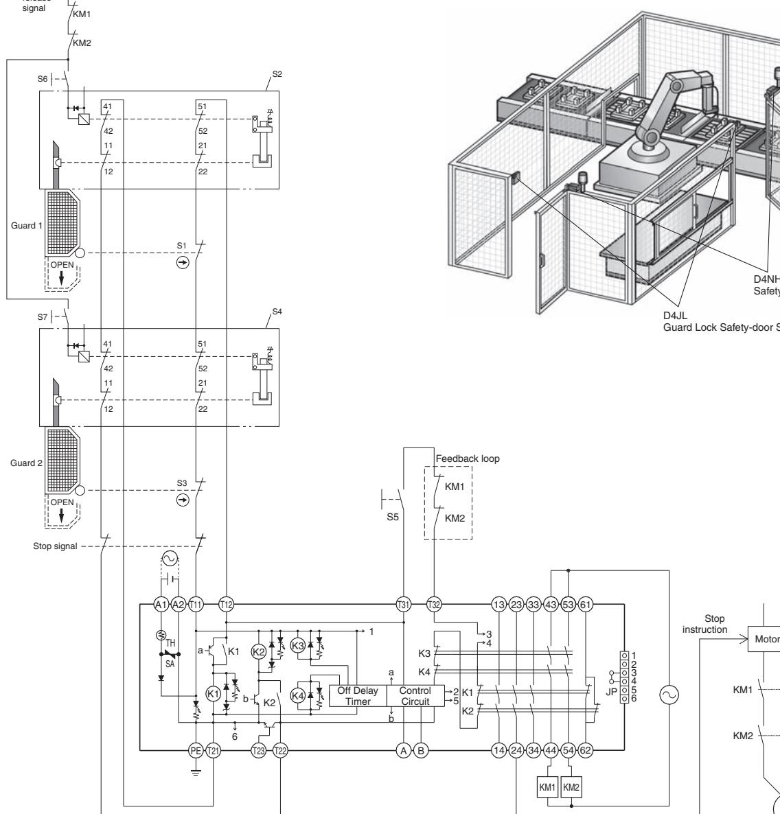
S1: Safety-door Switch with direct opening contact
