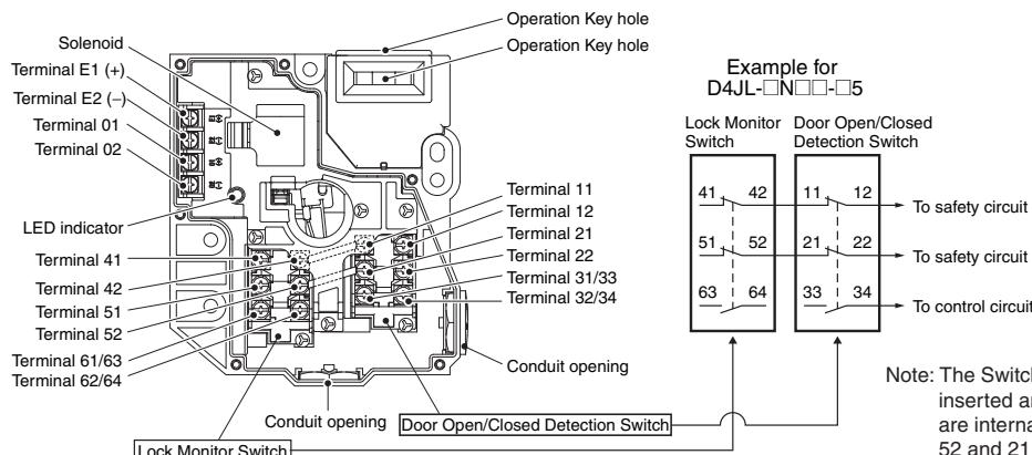
Note: The Switch is shown with the key inserted and locked. Terminals 42 and 11 are internally connected, as are terminals 52 and 21 (according to GS-ET-19).
