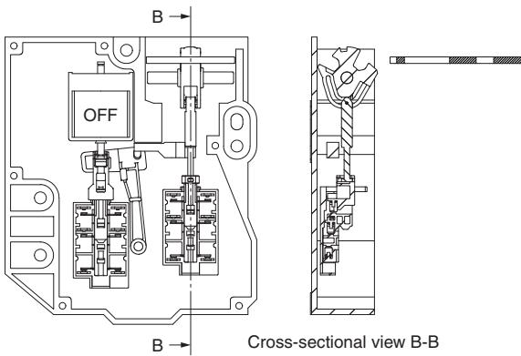
Operation Key inserted: Door locked.
