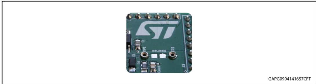
Figure 4: Mounting through-hole sense resistor
