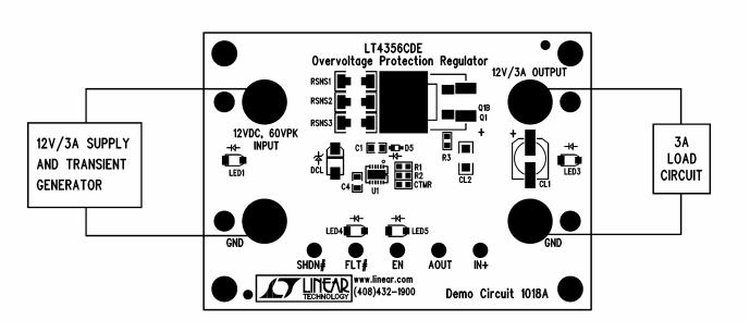
Figure 1: Proper Measurement Equipment Setup
