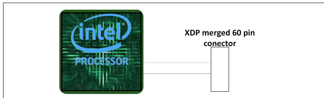
Figure 1-2. Merged XDP Connector for Processor and PCH
