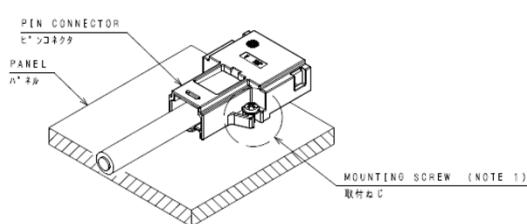
FIG.2 PANEL MOUNTING METHOD
