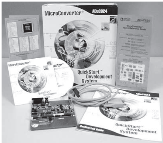
Figure 65. Components of the QuickStart Development System
