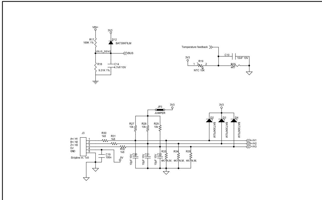
Figure 5: Schematic - Analog conditioning and Current protection circuit
