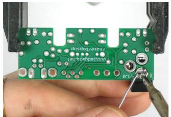
Flip over the PCB - you can either tape the DC jack down or use a finger to keep it place.
