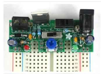
Now place the power supply on top. If it fits nicely, solder the four pins.
