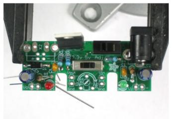
Finish off the 'low voltage' side by inserting the second 1.0K resistor **R2** and the second 0.1uF ceramic capacitor **C4**.
