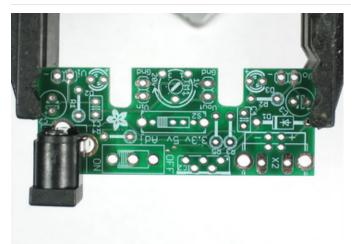
We'll start by placing the DC power jack. This is how we will attach outlet power supplies to the board. The jack is 2.1mm which is the most common size.
