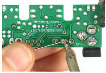
Tape or hold the switch in place while you solder all three pins.
