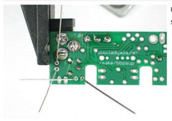
Bend the leads out so the parts sit flat against the PCB. Solder and clip the leads.
