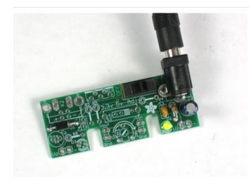
Lets take a break and test the current progress. Take the kit out of the vise and make sure there are no stray wires kicking around that could cause the board to short.
