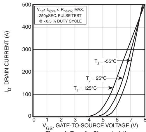
Figure 4, Transfer Characteristics
