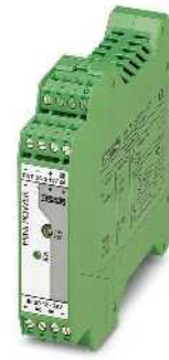
DC/DC converter, 12 - 24 V DC / 5 - 15 V DC, 2 A
