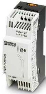
Power supply, 1 AC, 24 V DC, 0.75 A
