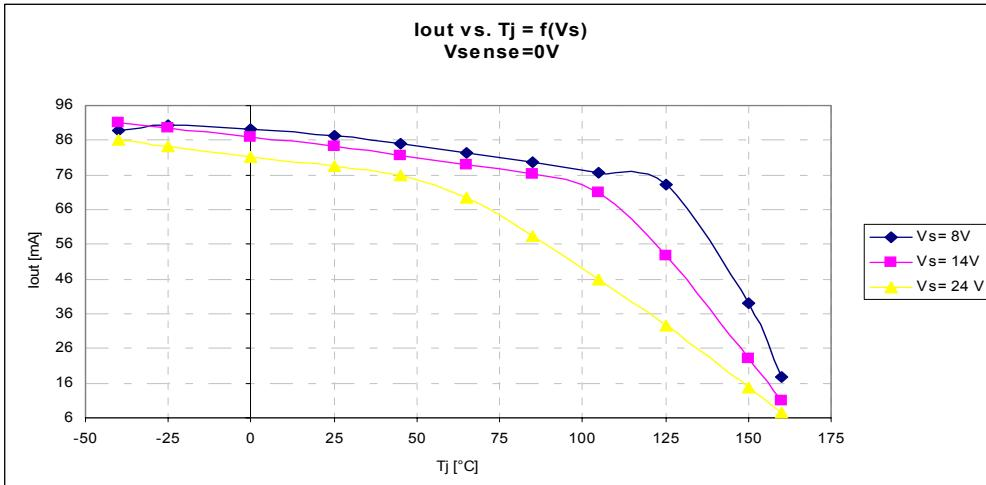
**Figure 7**  $I_{\text{out}}$  vs  $T_j = f(V_s)$
