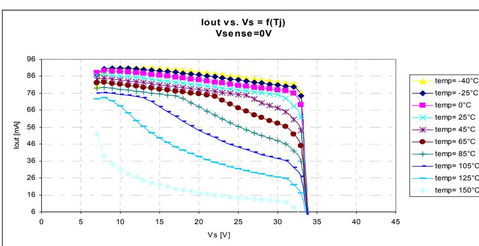
**Figure 8**  $I_{\text{out}}$  vs  $V_s = f(T_j)$
