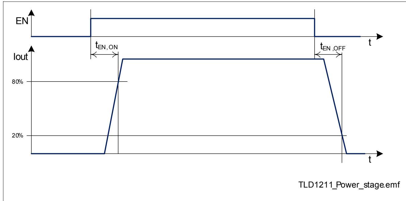
**Figure 4 Timing Diagram**
