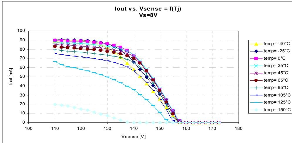
**Figure 9**  $I_{\text{out}}$  vs  $V_{\text{sense}} = f(T_j)$  at  $V_s = 8 \text{ V}$
