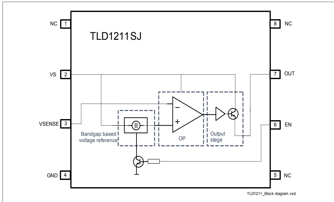
**Figure 1** Block Diagram
