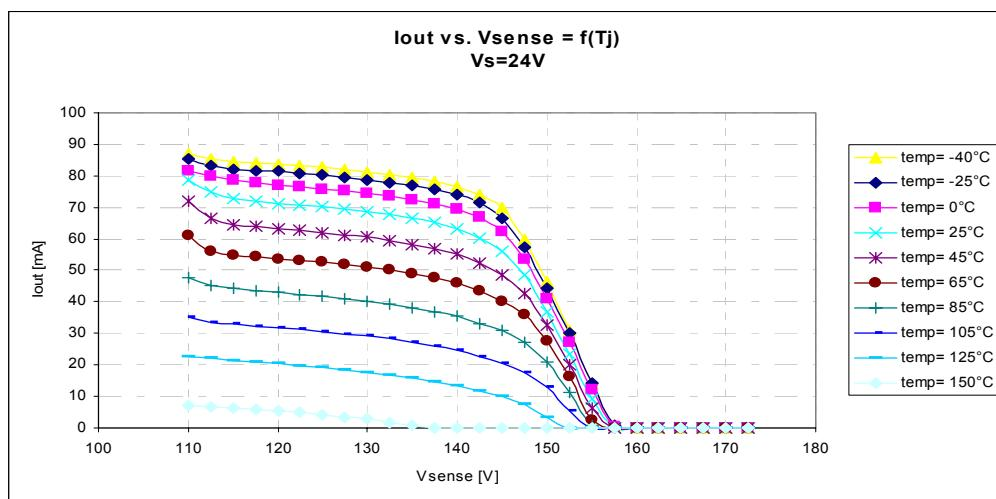
**Figure 11**  $I_{out}$  vs  $V_{sense} = f(T_J)$  at  $V_s = 24$  V
