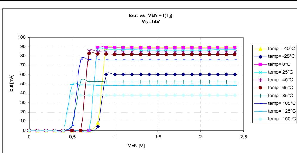
**Figure 12**  $I_{out}$  vs  $V_{EN} = f(T_J)$  at  $V_s = 14$  V
