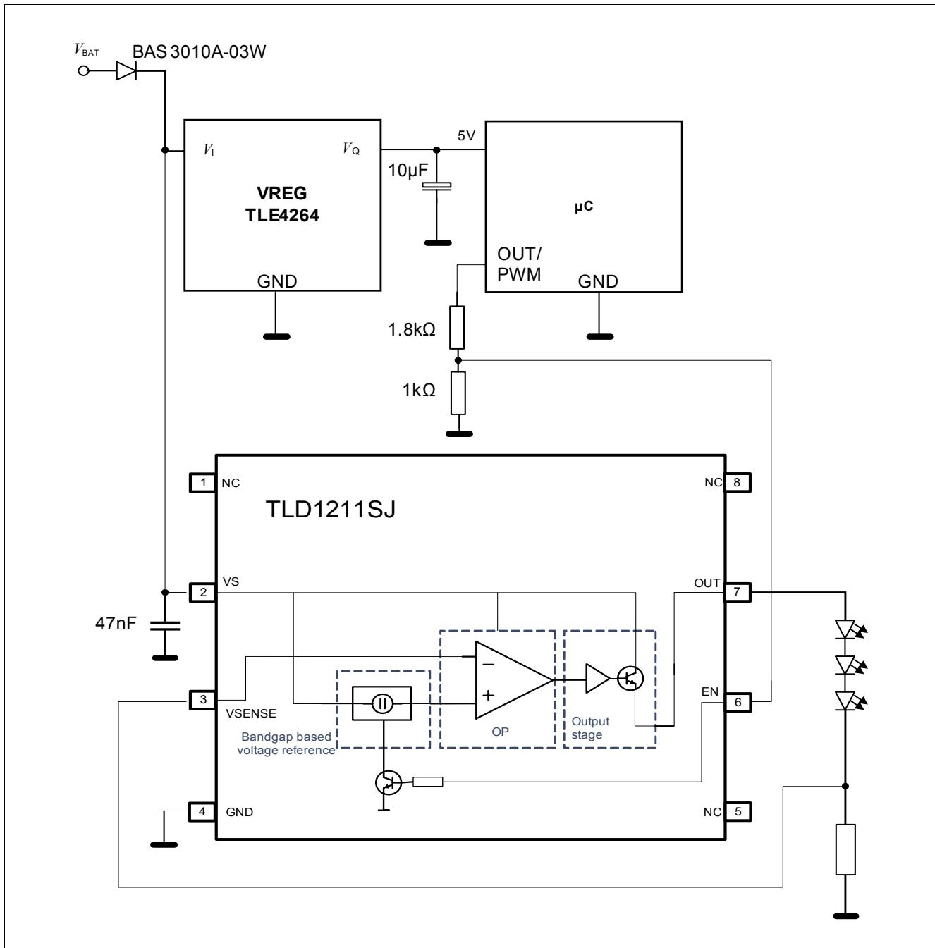
**Figure 17 Application Information with Integrated Output Stage Usage**
