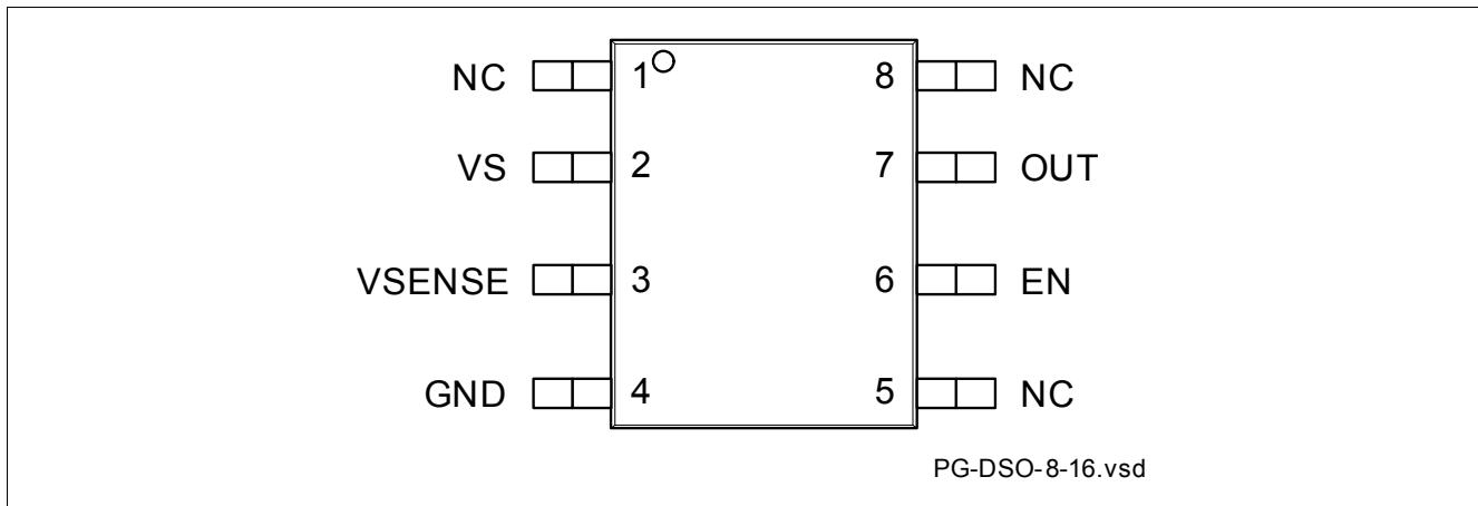
**Figure 3** Pin Configuration
