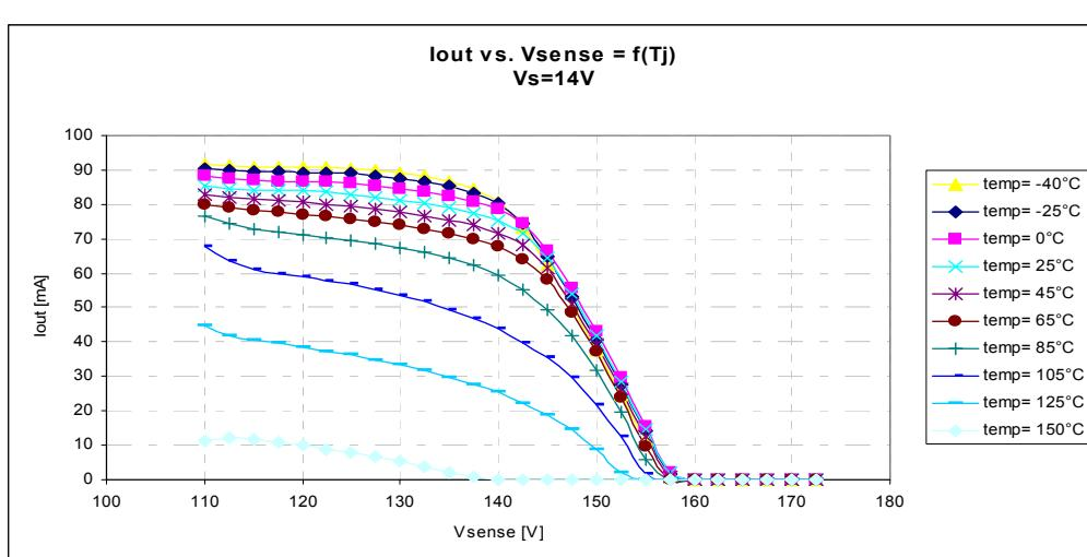
**Figure 10**  $I_{\text{out}}$  vs  $V_{\text{sense}} = f(T_j)$  at  $V_s = 14 \text{ V}$
