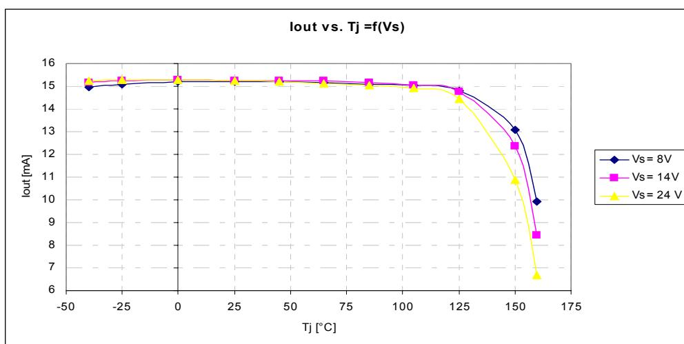
**Figure 5**  $I_{out}$  vs  $T_j$  =  $f(V_s)$
