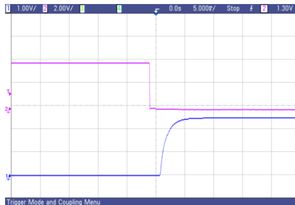
Fig. 64 AVO75-48S2V5 typical start-up from CNT on
