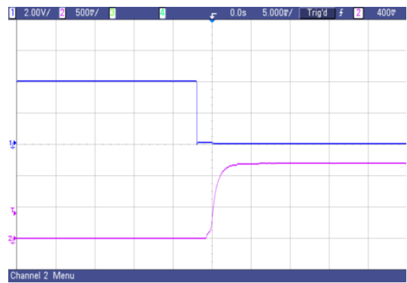
Fig. 58 AVO75-48S1V2 typical start-up from CNT on
