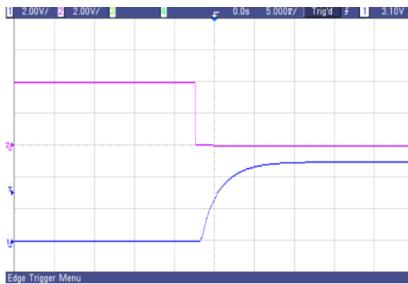
Fig. 68 AVO75-48S05 typical start-up from CNT on
