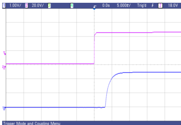
Fig. 63 AVO75-48S2V5 typical start-up from power on
