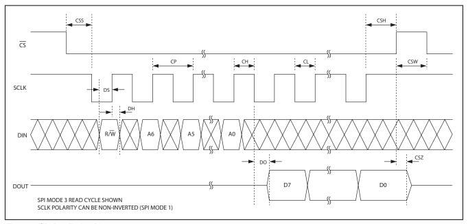
Figure 3. SPI Bus Timing Diagram
