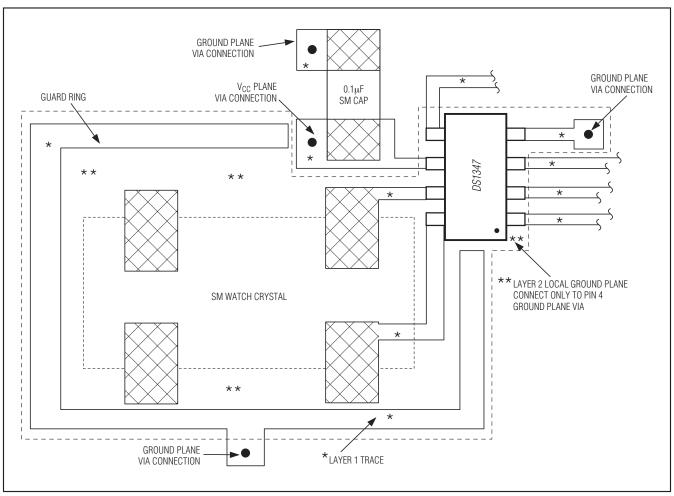
Figure 4. Crystal PCB Layout
