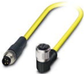
Sensor/Actuator cable, 4-position, PVC, Yellow RAL 1021, Plug straight M8, on Socket angled M12-SPEEDCON, A-coded, Cable length: 1.5 m
