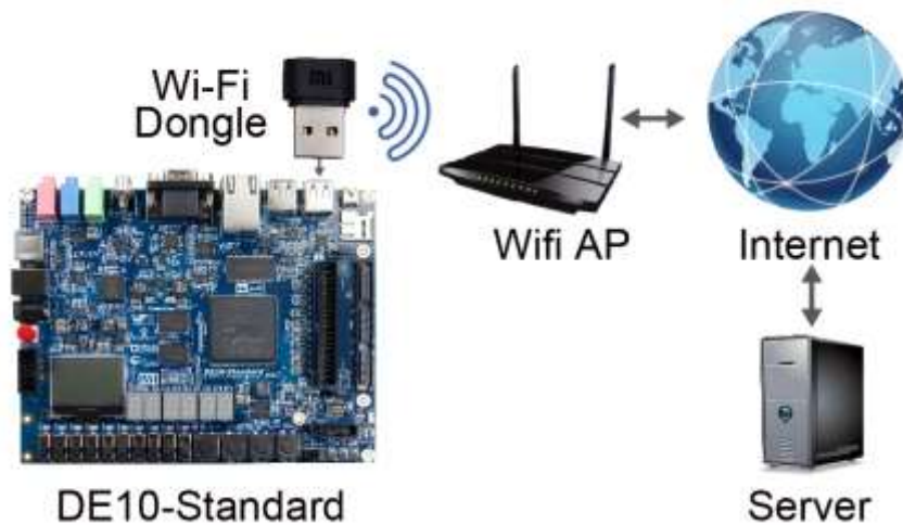
Figure 6-15 System diagram of USB Wi-Fi dongle
