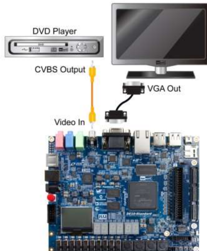
Figure 5-12 Setup for the TV box demonstration (VIP)
