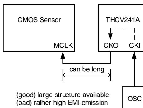
Figure 2. Reference clock supply clock buffer method (optional)
