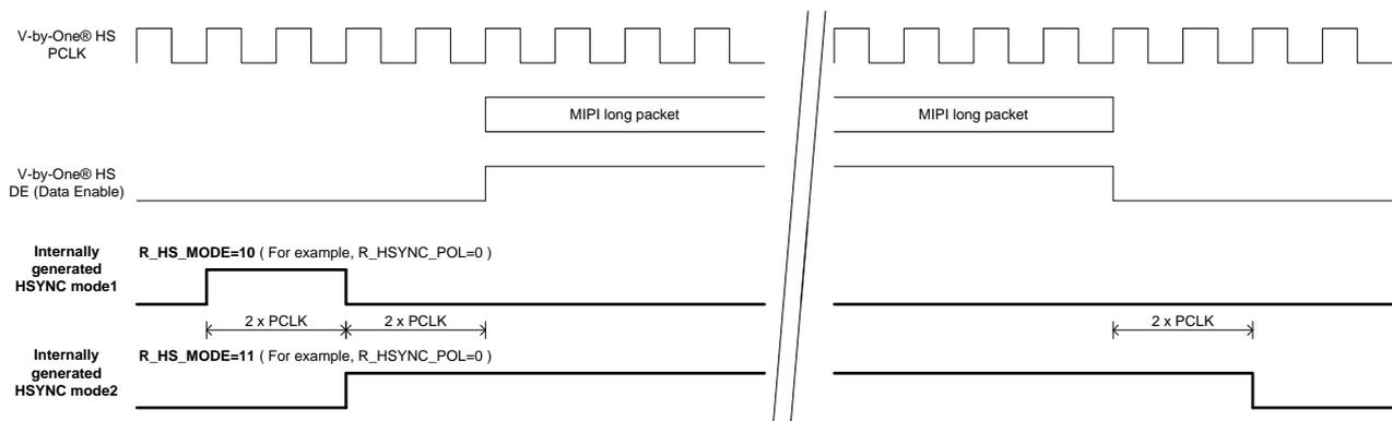
Figure 9. Internally generated HSYNC in Vertical active period
