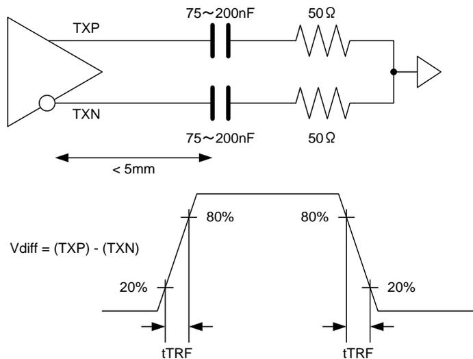
Figure 25. CML Transmitter t<sub>TRF</sub>
