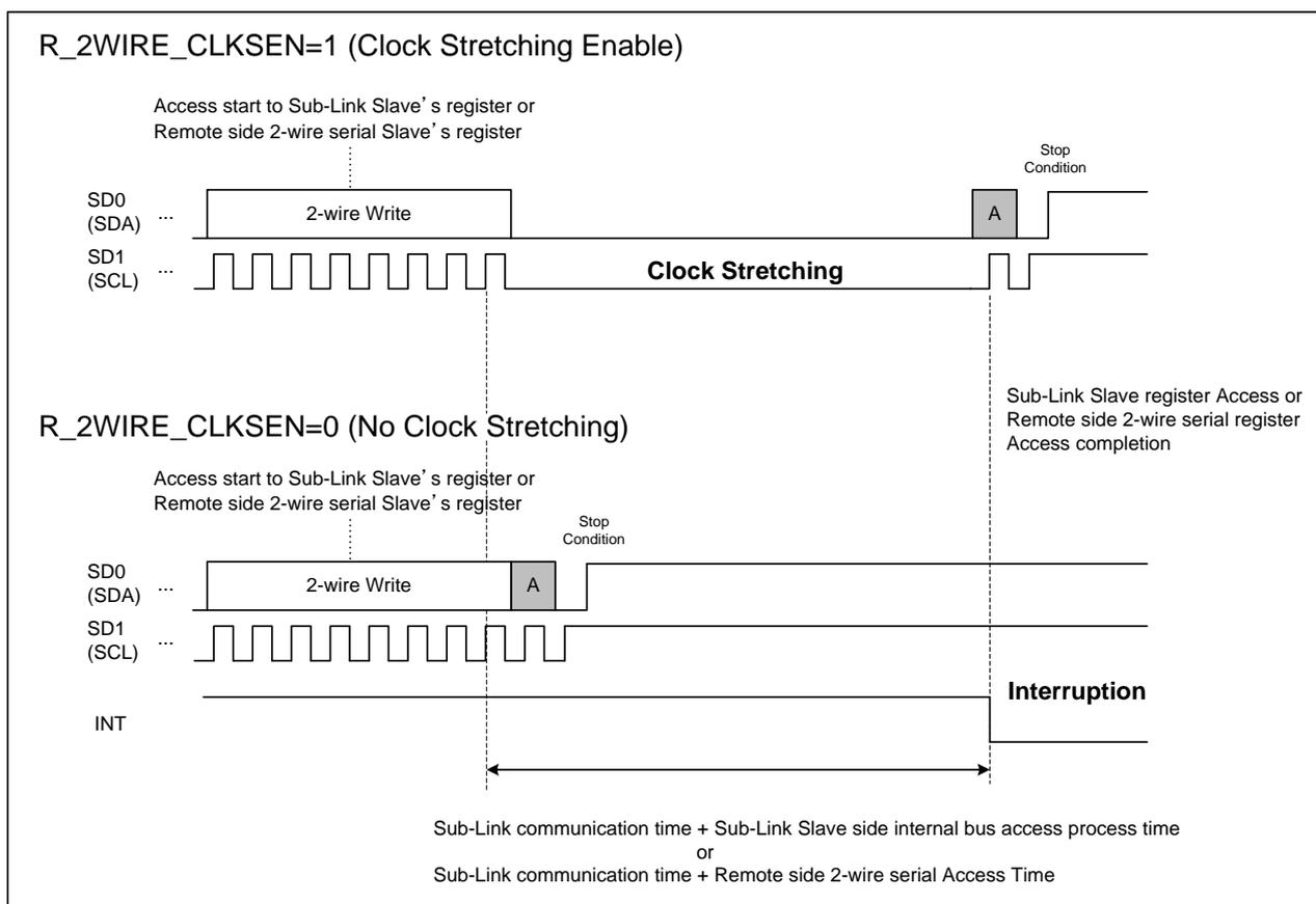
Figure 18. Sub-Link Master 2-wire slave clock stretching operation
