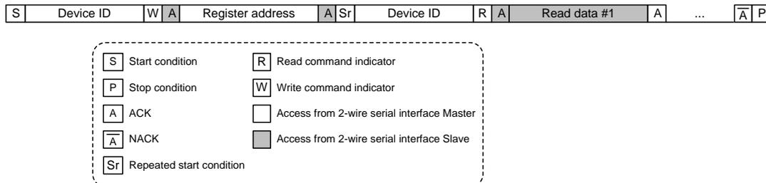
Figure 15. 2-wire serial I/F read to THCV241A local register protocol
