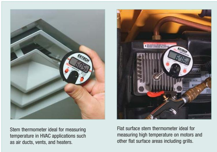
Stem thermometer ideal for measuring temperature in HVAC applications such as air ducts, vents, and heaters.
