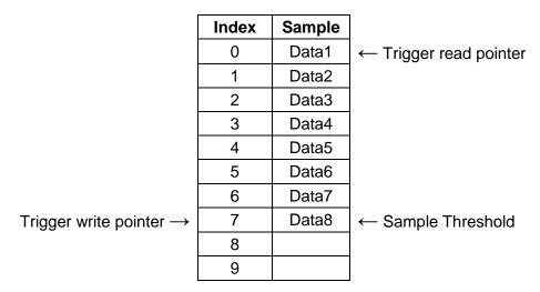
Figure 13. Additional Data Prior to Trigger Event
