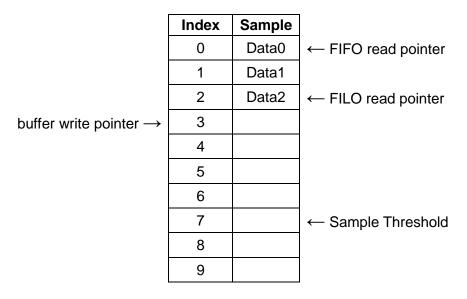
Figure 10. Buffer Filling
