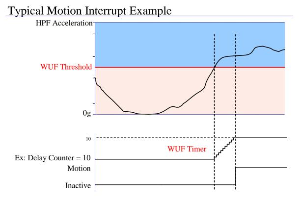
Figure 4. Latched Motion Interrupt Response
