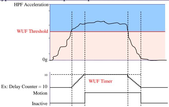
Figure 5. Unlatched Motion Interrupt Response
