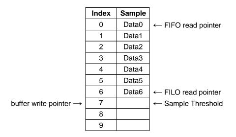
Figure 11. Buffer Approaching Sample Threshold
