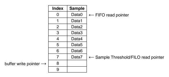
Figure 12. Buffer at Sample Threshold
