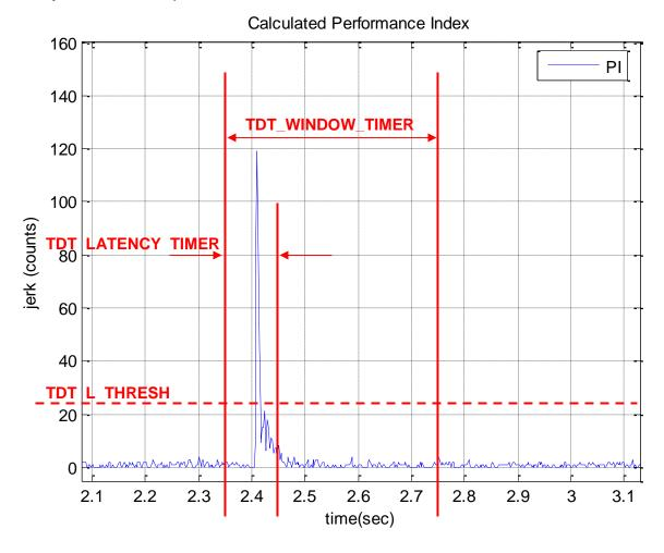
Figure 7. Single Directional Tap<sup>™</sup> Timing
