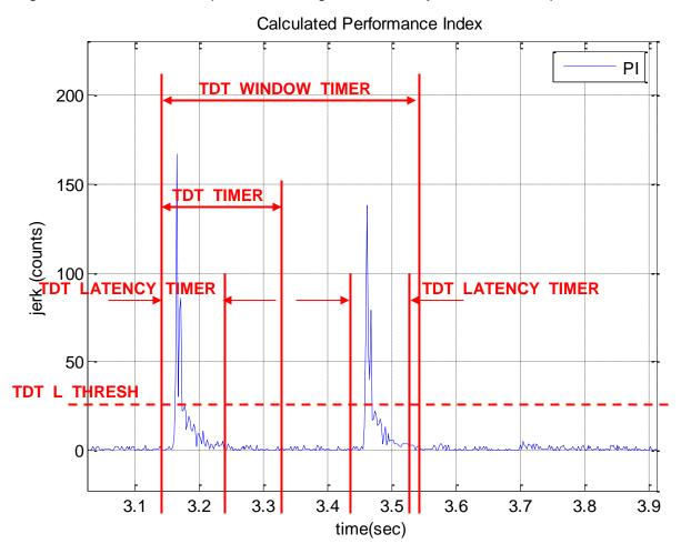
Figure 8. Double Directional Tap<sup>TM</sup> Timing
