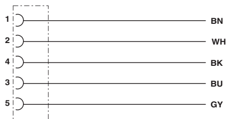
Contact assignment of the M12 socket
