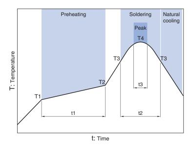
Soldering Preheating Peak Temp. Temp. Time Temp. Time Time T1 T2 T4 Т3 150°C 180°C 60 to 120s 230°C 10 to 30s 245°C 5s max.
