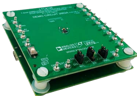
Figure 7. DC2662A mounted on top of DC2661A
