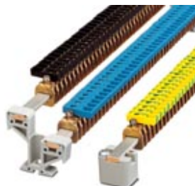
Power terminal block, Connection method: Screw connection, Cross section: 0.5 mm 2 - 6 mm 2 , AWG 20 - 10, Width: 7 mm, Height: 23.6 mm, Color: green-yellow, Mounting type: Neutral busbar
