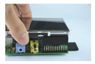
**NOTE:** The 4DPi-32 is supported only by the 26 way header, and therefore pressing on the touch screen may result in the 4DPi-32 moving towards the Raspberry Pi, and therefore the circuitry touching the Raspberry Pi. This could result in damage to either product if a short circuit were to occur. It is therefore highly encouraged to mount the display and attach the Pi to the mounted display.
