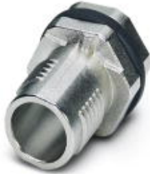
M12-SPEEDCON housing screw connection for M12 male inserts, with flat gasket, for all Speedcon-compatible THR and wave soldering contact carriers
