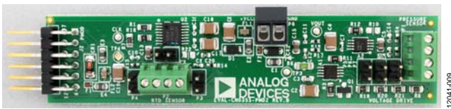
Figure 9. Photo of EVAL-CN0355-PMDZ Board
