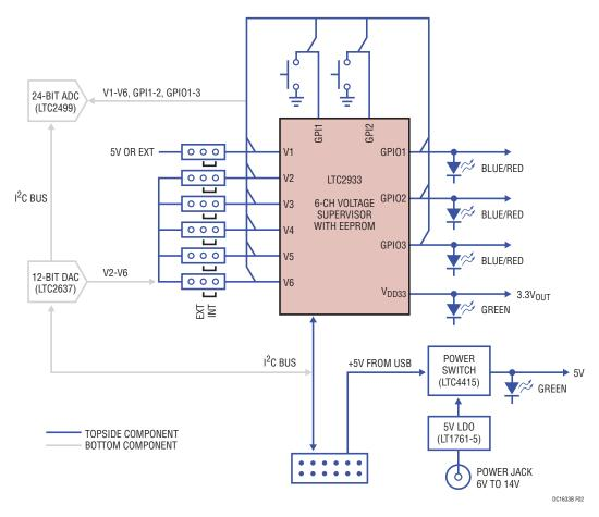
Figure 2. Simplified Block Diagram of the DC1633B
