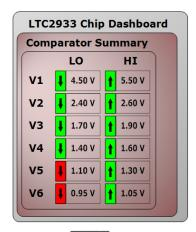
has been programmed to function as MARG, enabling the LTC2933 to ignore all UV conditions. Notice that when the pushbutton is depressed, GPIO3 returns high (blue). This is useful when the system does not want to be informed of a UV condition during margin low testing. Moving the DAC voltages back to 1.2V and 1V returns GPIO3 to a high state (blue), indicating there is no UV condition.
