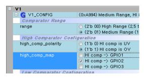
2. Configure GPI1 as a Manual Reset. Map GPI1 to GPI01.
