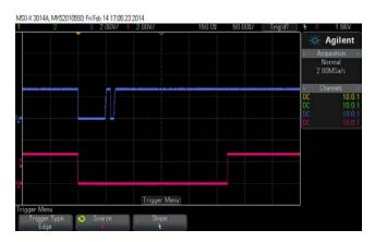
When configured in this way, GPIO1 provides a system reset for the host processor and GPI1 can drive a system reset (GPIO1) with a push of a button. You may set the GPIO1 delay-on-release time to 410ms to experience the extended reset firsthand. The UV condition indicator remains on GPIO3. The OV condition is indicated as a latched ALERT on GPIO2. When the GPI1 pushbutton is pressed, a system reset is asserted on GPIO1 and the ALERT is released if the OV condition is removed.
