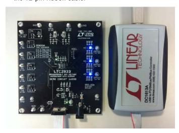
Figure 4. Connecting DC1633B Board and the DC1613 USB to I<sup>2</sup>C/SMBus/PMBus Controller
