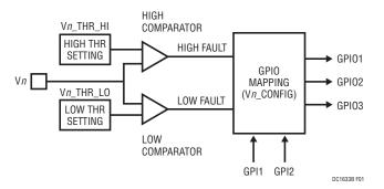
Figure 1. Simplified Block Diagram of Voltage Supervisor Input
