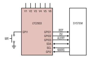
1. To program GPIO1 to system reset function, first uncheck the mapping of all V1-V6 channels to GPIO1.
