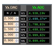
the DAC output by clicking the up/down arrows on the individual DAC box or by double-clicking the DAC value and entering a new value in the box. V5 and V6 will report a UV, turning the LED on
