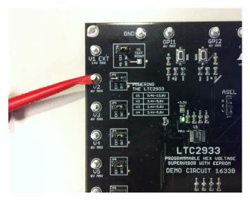
Apply an external supply voltage to the turret. It is recommended to drive V1-V4 turrets with a low impedance ( $<10\Omega$ ) voltage source. A sensor or other moderate source impedance voltage may be supervised on V5 or V6 inputs. A battery voltage may be supervised on V1-V4 and power the chip since the LTC2933 supply current is  $<700\mu$ A.
