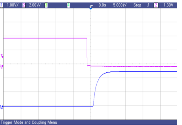
Fig.64 AVO50-48S2V5 typical start-up from CNT on
