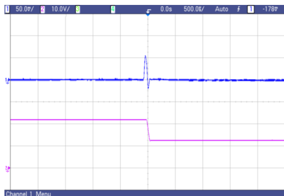
Fig.34 AVO505-48S2V5 typical transient response to step decrease in load from 50% to 25% of full load, room temperature, 48Vdc input ( \Delta I_o/\Delta t = 0.1A/1\mu s )
