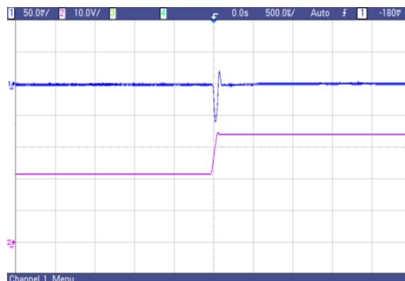
Fig. 35 AVO50-48S2V5 typical transient response to step increase in load from 50% to 75% of full load, room temperature, 48Vdc input ( \Delta I_o/\Delta t = 0.1A/1\mu s )
