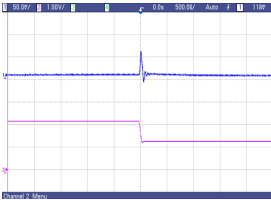
Fig.22 AVO50-48S1V2 typical transient response to step decrease in load from 50% to 25% of full load, room temperature, 48Vdc input ( \Delta I_o/\Delta t = 0.1A/1\mu s )
