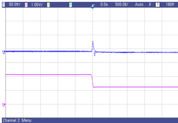
Fig.30 AVO50-48S1V8 typical transient response to step decrease in load from 50% to 25% of full load, room temperature, 48Vdc input ( \Delta I_o/\Delta t = 0.1A/1\mu s )
