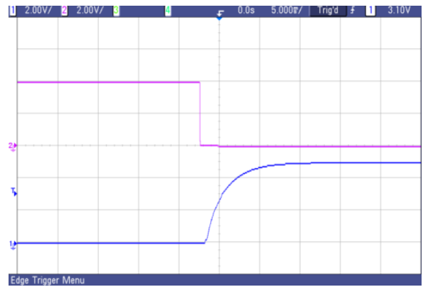
Fig.68 AVO50-48S05 typical start-up from CNT on
