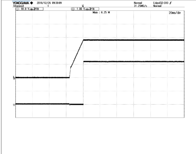
Figure 9: PG voltage vs. Vout @ Vin=220Vac, 0Alout TOP: Vout, 10V/div, 20mS/div BOTTOM: PG, 1V/div, 20mS/div
