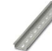
DIN rail, material: steel galvanized and passivated with a thick layer, perforated, height 7.5 mm, width 35 mm, length: 2000 mm
