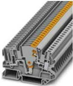
Test disconnect terminal block, Connection method: Screw/plug-in connection, Cross section: 0.14 mm<sup>2</sup> - 6 mm<sup>2</sup>, AWG: 26 - 10, Width: 6.2 mm, Color: gray, Mounting type: NS 35/7,5, NS 35/15
