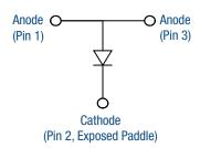
Figure 1. CLA4610-085LF Block Diagram
