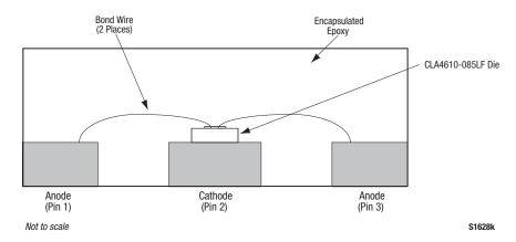
Figure 5. Cross-Sectional View of the CLA4610-085LF
