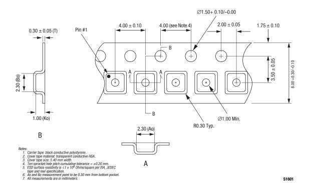
Figure 10. CLA4610-085LF Tape and Reel Dimensions
