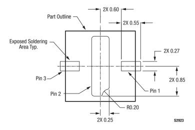
Figure 7. CLA4610-085LF PCB Layout Footprint
