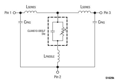
Figure 6. CLA4610-085LF Electrically Equivalent Circuit
