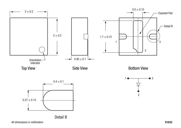
Figure 9. CLA4610-085LF QFN Package Dimension Drawing
