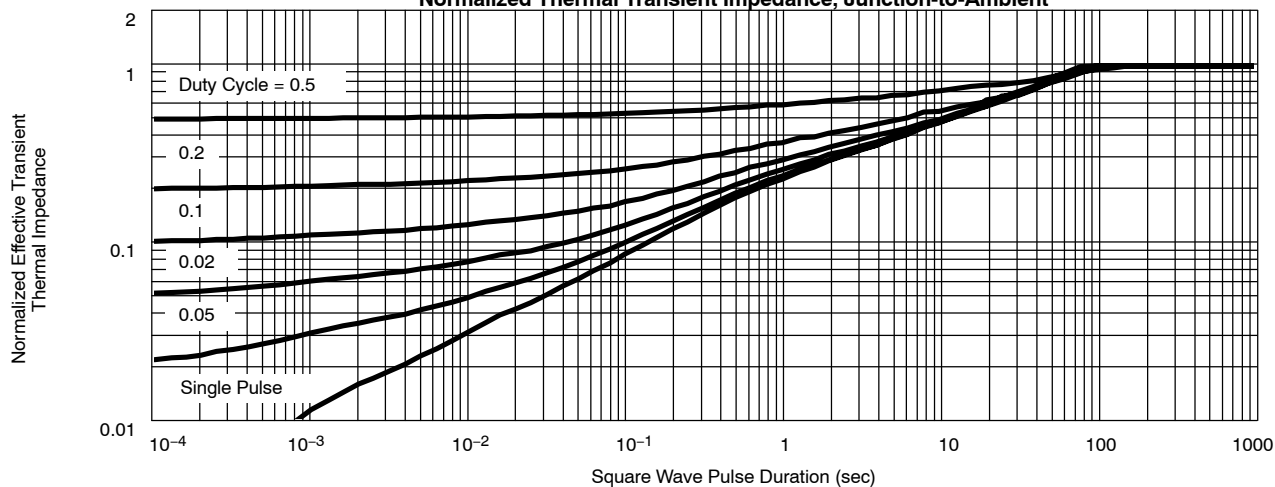
Normalized Thermal Transient Impedance, Junction-to-Case
