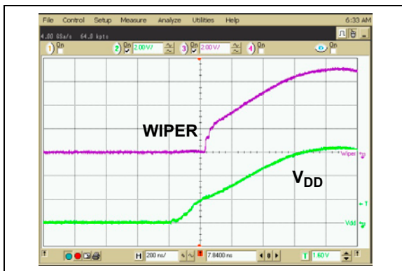
FIGURE 2-52: 50\text{ k}\Omega – Power-Up Wiper Response Time.
