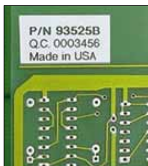
Circuit board labeling
