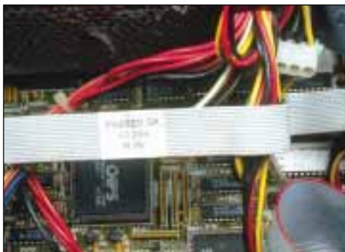
Flat Ribbon Cable Labeling
