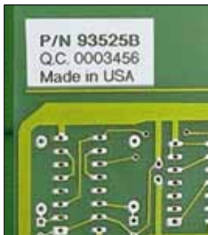
Circuit board labeling
