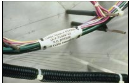
Identify harness board assemblies
