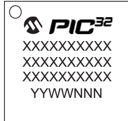
64-Lead TQFP (10x10x1 mm)
