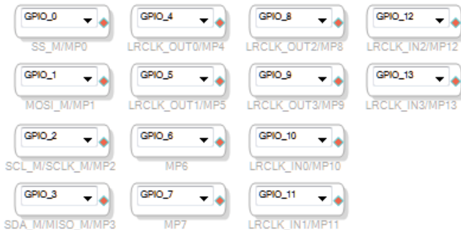
Figure 76. Complete Set of General-Purpose Inputs in SigmaStudio
