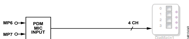
Figure 45. PDM Microphone Input Mapping to DSP in SigmaStudio
